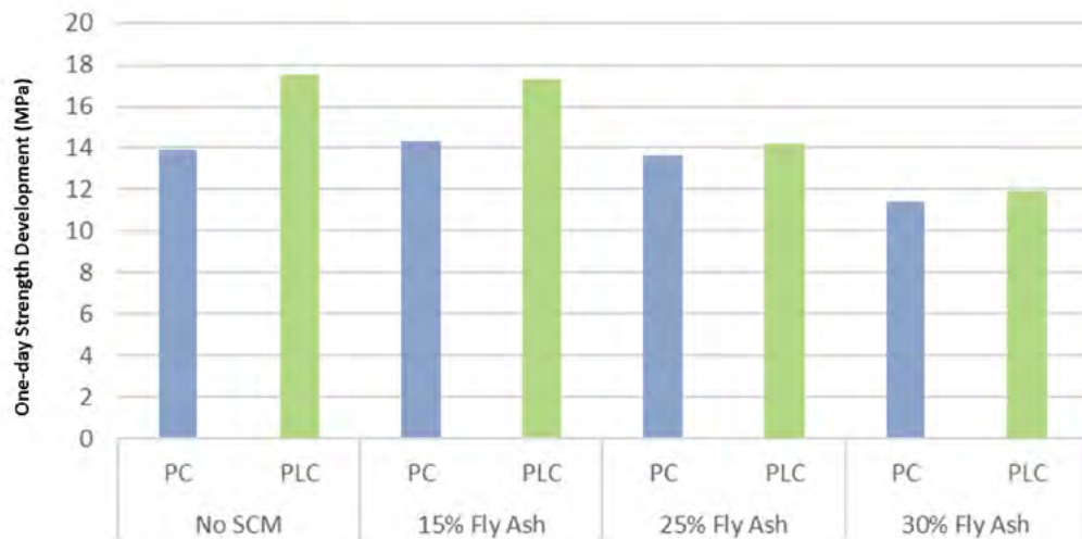
Figure 7: High early strength gain in PC and PLC concrete (Tennis et al. 2011)
